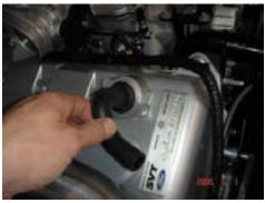
106. Attach the supplied vacuum line from the turbo compressor to the underside of the wastegate.
