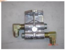
116. Install adapter onto engine and tighten
