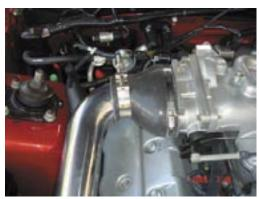
103. Bolt Blow Off Valve to Stub off of inlet tube. Install blow off valve outlet to stub on the 4-inch tube inlet, using 1 3/8 silicone hose and supplied clamps.
