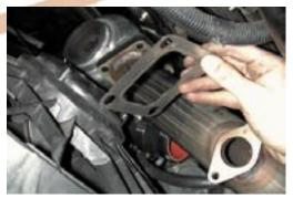
63. P/S line will need to be bent towards engine to make clearance for down pipe.
