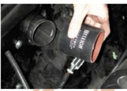
100. Install 4"turbo inlet pipe, Massair meter, and filter onto turbo inlet. Make sure that the flow is correct and the air filter is secured to the end of the meter. Leave clamps loose until final intercooler pipe fitment.
