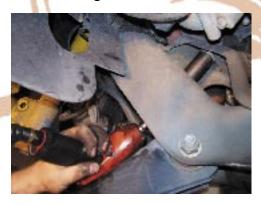
18. Support engine and transmission with appropriate upper support tool or support from beneath.
