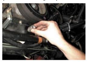
58. Next, take a 3/8" pipe tap (supplied) and coat it with grease. Tap hole in pan. The grease will catch the tapped shavings.
