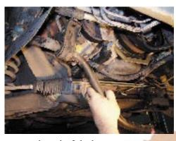
4. Remove steering shaft bolt
