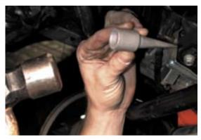
56. Mark a point <sup>3</sup>/<sub>4</sub>" Inches down from oil pan rail, and centered left to right.
