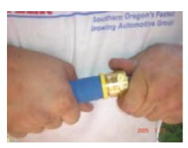
122. Install and tighten oil lines, \*note inlet and outlet\*
