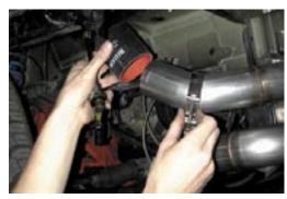
99. Install intercooler pipe #3 and silicone hose.
