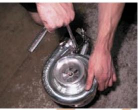
52. Install turbo support bracket to Cylinder Head using supplied M8x30mm socket head bolts and spacers.
