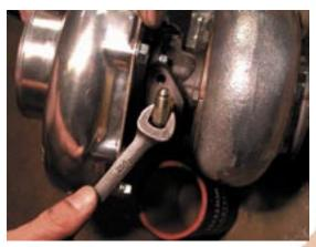
49. Install 90 degree barb fitting to compressor housing. Position fitting so it faces downwards. This will be connected to the underside of the wastegate.
