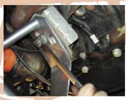
28.Install grease boots on lower ball joints
