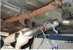
75. Bolt Y-pipe to mufflers.
