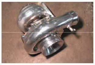
48. Install 90 degree 1/8 pipe to #4 fitting to top of turbo. Install and tighten fitting so it faces the rear of the car. (use minimal pipe paste)
