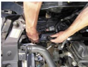
42. Reconnect (5) connectors through air inlet hole. This will open up the smaller hole in the fender, allowing installation of boost inlet tube.
