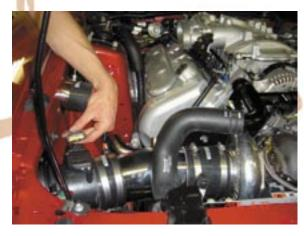
102. Install intercooler pipe #4 and 2.5" by Oval silicone hose adaptor to throttle body.
