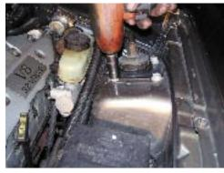
32.Remove plate from strut by removing large nut on top of strut shaft
