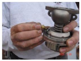
66. Install wastegate, using supplied gasket and bolts. Bolt wastegate to inlet pipe with supplied 8mm socket head bolts. There is no gasket between wastegate and the main pipe. Bolt wastegate outlet pipe to wastegate using gasket and supplied 5/16" socket head bolts. Leave bolts loose.
