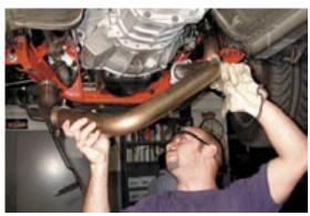
69. Bolt exhaust hanger to driver side transmission mount using supplied 5/16" bolt, nut and washer. This is the sheet metal bracket that is attached to the floor of the car.
