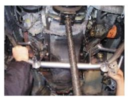
25.Install bushings and sleeves into tubular A-arms, making sure that the short sleeve is in front, and the long sleeve in back
