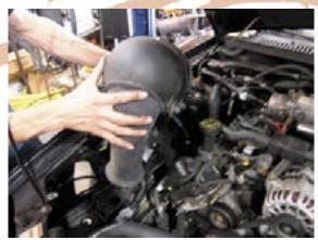
41. Disconnect (5) connectors and push harness through hole back into fender well.
