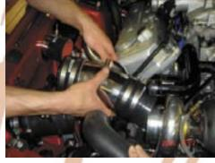
101. Re connect mass air meter, and plug in air temp sensor inside inner fender.
