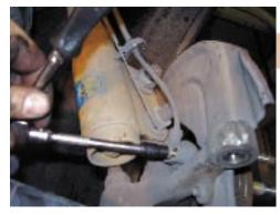
13.Loosen lower ball joint 15/16 nut (both left and right) until there is a 1/8 inch gap with the nut maintaining full thread engagement.
