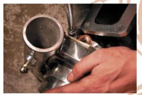
51. Slide supplied 2 ½" silicone hose onto end of compressor housing. Install and tighten supplied 2 ½" T-bolt clamp.
