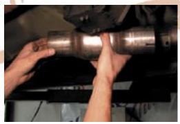
74. Install Y-pipe onto straight pipe or cat, sliding clamp on first. If desired, Install O2 sensors. If rear O2 sensors are to be used, extending the factory harness by cutting & soldering the wires will be necessary.
