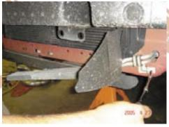
91. Relocate PS cooler line clip to other slot in radiator support.
