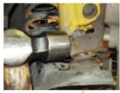
15. Support A-arm with jack to take load off of spring and remove the 2 strut to spindle bolts, then lower A-arm, being cautious because spring is under pressure.
