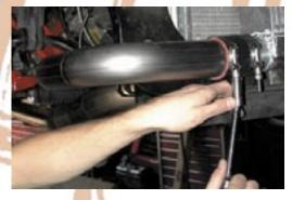
97. Install intercooler pipe #2 onto upper intercooler outlet.
