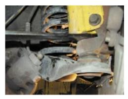
14.Use an air hammer or electric hammer with a pickle fork in order to disengage ball joint from spindle
