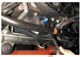
61. Install main turbine inlet pipe. From underneath, raise pipe up and bolt to passenger side exhaust manifold using factory nuts.
