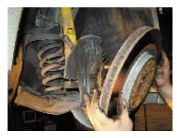
12. Remove ABS sensor lines both left and right
