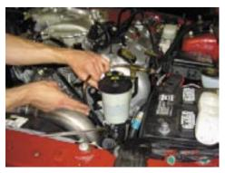
64. Hang down pipe to exhaust housing using supplied V-band clamp. Leave clamp loose. (Heat shield not shown with pic)
