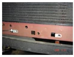
92. Install intercooler with supplied metric bolts. Bolt it to lower radiator support, leaving bolts loose.
