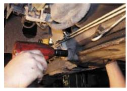
6.Remove steering tie rod ends (you may want to try using an air hammer with a pickle fork to remove the tie rod end if it is difficult to remove)
