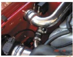
104. Position all intercooler pipes and tighten all clamps. 105. The next step is to connect the valve covers to the 4" inlet. Take supplied 3/8 hose and connect it to the PCV valve on the driver side valve cover. Route 3/8 line to supplied 3/8X1/2X1/2 tee and connect tee to the small hose on the passenger side valve cover. Next connect 3rd leg of tee to the ½" stub on the polished 4" inlet pipe.
