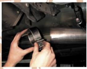
73. Install straight pipe or catalytic converter onto the "double barrel". Again, slide clamp on first.
