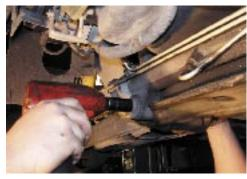
6.Remove steering tie rod ends (you may want to try using an air hammer with a pickle fork to remove the tie rod end if it is difficult to remove)
