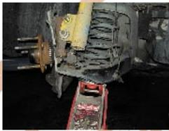
16.Remove spindle, both left and right
