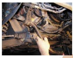
4.Remove steering shaft bolt
