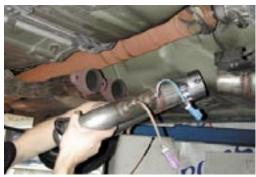
75. Bolt Y-pipe to mufflers.
