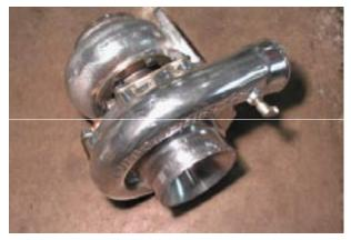
48. Install 90 degree 1/8 pipe to #4 fitting to top of turbo. Install and tighten fitting so it faces the rear of the car. (use minimal pipe paste)
