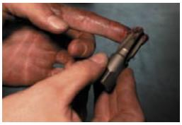
59. Remove tap and wipe the remaining grease from hole, being careful not to let shavings fall into pan. 60. Take supplied 3/8" pipe to #10 fitting and install in pan using pipe paste to seal threads.
