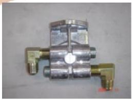
116. Install adapter onto engine and tighten
