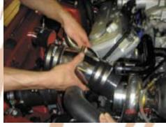
101. Re connect mass air meter, and plug in air temp sensor inside inner fender.
