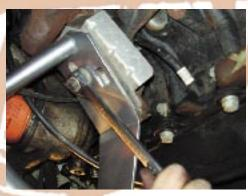
28.Install grease boots on lower ball joints
